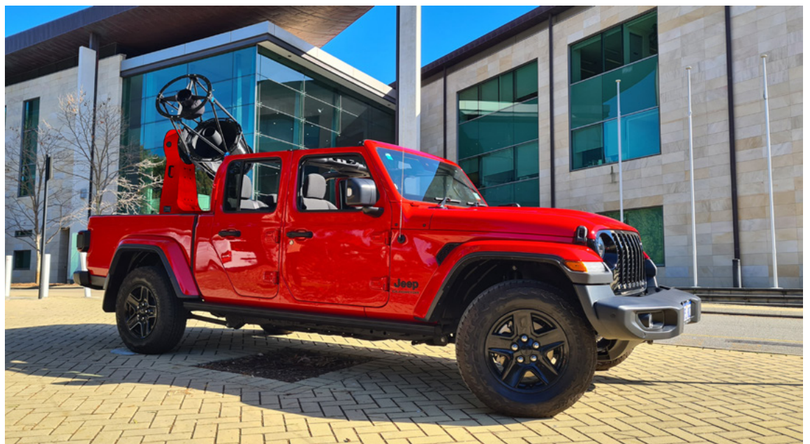
Jeep-mounted transportable free-space optical communications terminal from the Teranet free-space optical communications ground station
